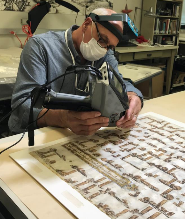
Figure 1: Christopher Foster using an x-ray fluorescence spectrometer to analyze the elemental composition of the pigments on the Qur'an folio (DIA 30.317, City of Detroit Purchase).
