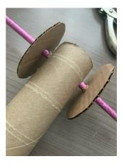
4. **Use a ruler to measure two holes for the back wheels and axle.** They should line up with the front end. Use your hole punch to punch two matching holes on the back end.
