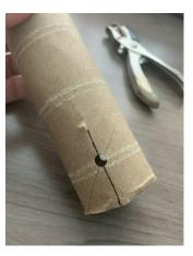
2. **Enlarge the holes.** Use a jumbo paper clip to enlarge the axle holes in the paper towel roll. If you only punch a pencil through the hole, it will be too tight to turn freely. Where the pencils fit into the wheels needs to be a tight fit. Where the pencil goes through the tube/body needs to be a loose fit. (It seems obvious, but it can be a common design problem).
